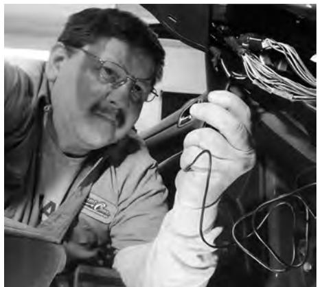
Ron Siekierke, a technician at Extreme Clean Automobile Detailing in Oshkosh, installs an IID.
